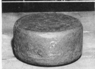
This radius was formerly machined on the blocks after they were reshaped in Blacksmith Shop. The forged blocks are now sent directly to the Hardening Room. A finished block is shown in the inset picture.
