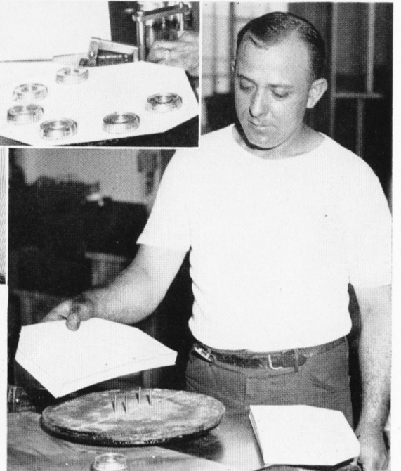
Thousands of scrap pieces of blotting paper used by the Lacquer Room were piling up after cutting full size blotters for taking excess shellac from fuse rings, until Tom Serendi, a battery captain, devised the shown turntable with four pins. Two holes were punched in the scraps. The pictures tell the story.
