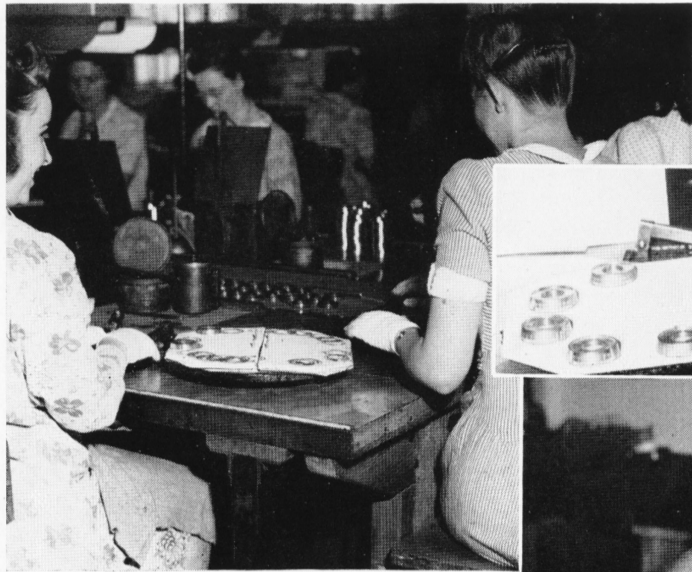
Thousands of scrap pieces of blotting paper used by the Lacquer Room were piling up after cutting full size blotters for taking excess shellac from fuse rings, until Tom Serendi, a battery captain, devised the shown turntable with four pins. Two holes were punched in the scraps. The pictures tell the story.
