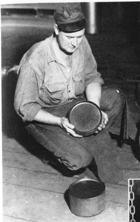
Tom Kaukas, Blacksmith Shop, is shown with his prize-winning forging die. This enables him to place a radius on dummy blocks used in the Extruded Rod Mill, when reshaping these blocks under the Forging Press.
